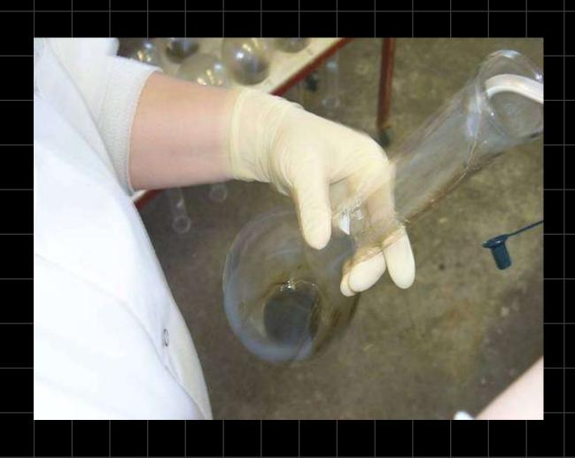
Manure added to flask and cylinder re-weighed to determine sample wt.
