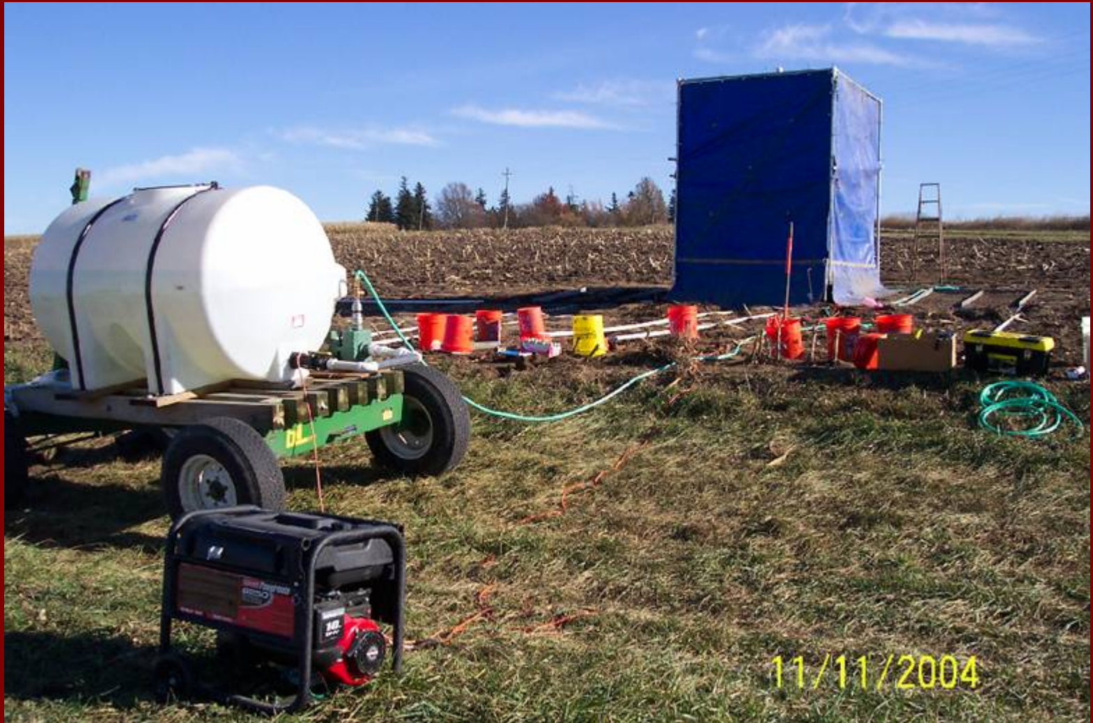
Field setup: Generator, 500 gallon tank, pump, rainfall simulator
